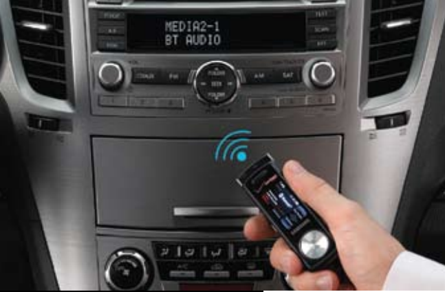
Bluetooth streaming audio, as shown in this Subaru Outback, allows the user to send music wirelessly from a compatible cell phone to the car's audio system.
